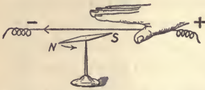
FIG. 317. — The Thumb Shows the Direction in Which the N-Pole Moves.
